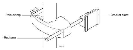
The cable-head bracket can be adjusted four ways:
