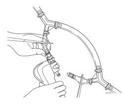
4 Unclamp the Shunt Bypass Lines and start the pump to circulate prime solution through the shunt sensor. Prime and debubble CDI Shunt Sensor and the Shunt Bypass Line, inspecting the line and CDI Shunt Sensor for bubbles. Verify that the cable-head is sufficiently supported and that the tubing is not kinked.
