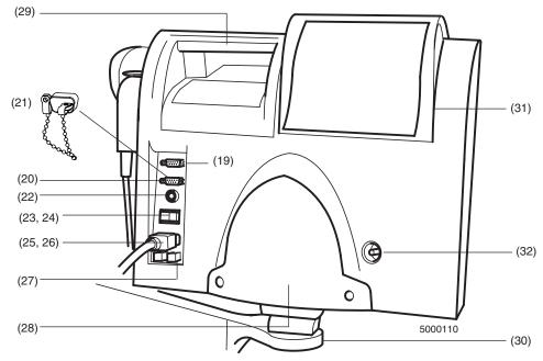
This figure shows the back panel of the monitor.
