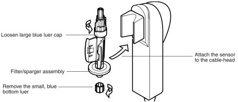
10 Using sterile technique, fully loosen the large, blue top venting luer cap on the sensor(s).
