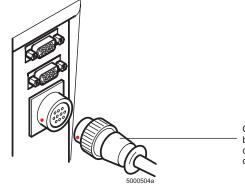
Connect the calibrator cable to the monitor by aligning the red dots on each of the connectors and pushing the calibrator cable connector onto the monitor connector.
