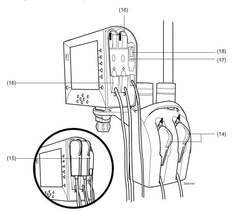
(14) Arterial and/or venous blood parameter module (BPM) cable-heads. Modules for monitoring pH, PCO<sub>2</sub>, PO<sub>2</sub>, potassium and temperature.
